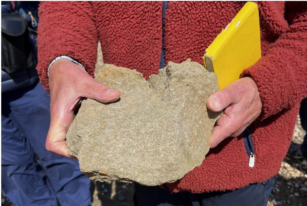
Figure 6 Glauconitic sandstone from the Ferruginous Sand Formation.
